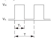
$V_{IH} = 4.75 \text{ to } 5.25 \text{ V} \quad V_{IL} = 0 \text{ to } 0.4 \text{ V} \\ PWM \text{ duty cycle (\%)} = \frac{T_1}{T} \times 100 \qquad PWM \text{ frequency } 25 \text{ (kHz)} = 0.00 \text{ (kHz)}$ Current source (Isource) = 1 mA max. (when control voltage is 0 V) Current sink (Isink) = 1 mA max. (when control voltage is 5.25 V) Control terminal voltage = 5.25 V max. (when control terminal is open)
