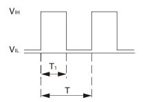
$V_{IH} = 2.8 \text{ to } 10.5 \text{ V} \qquad V_{IL} = 0 \text{ to } 0.5 \text{ V}$   $PWM \text{ duty cycle } (\%) = \frac{T_1}{T} \times 100 \qquad PWM \text{ frequency } 1 \text{ (kHz)} = \frac{1}{T}$  Current source (Isource) = 5 mA max. (when control voltage is 0 V) Current sink (Isink) = 0.1 mA max. (when control voltage is 10 V) Control terminal voltage = 11.5 V max. (when control terminal is open)
