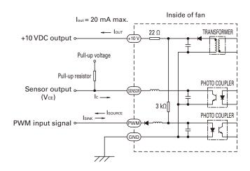
$$\begin{split} &V_{\text{CE}} = +27.6 \text{ V max.} \\ &I_{\text{C}} = 10 \text{ mA max.} \left[ V_{\text{OL}} \!\!=\!\! V_{\text{CE}} \left( \! \text{SAT} \right) \!\!=\!\! 1 \text{ V max.} \right] \\ &Pull-up \ resistor = 5 \ k\Omega \ max. \end{split}$$
