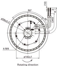
Power lead wire AWG 20 UL 1430 Other lead wire AWG 24 UL 1430
